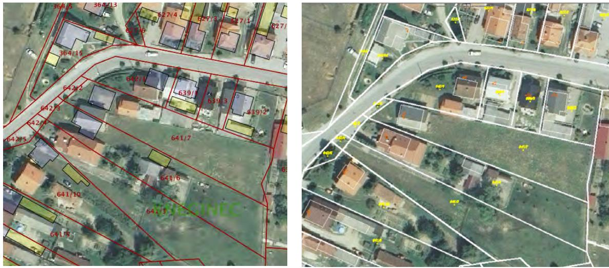
Figure 1. DCM overlapped on DOP before and after improvement
